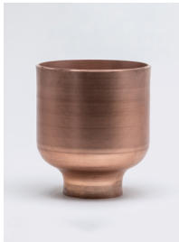
DED, WEBAM (Wire Electron Beam Additive Manufacturing) Wire process
